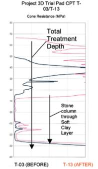
The use of Vibro-Stone Columns permitted the construction of an additional coal Stacker and coal stockyard on soft mangrove clays.
