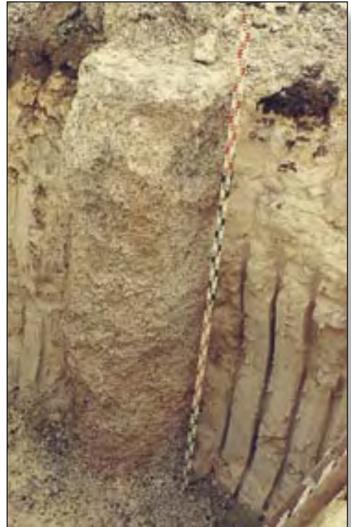
Excavated grouted stone column
